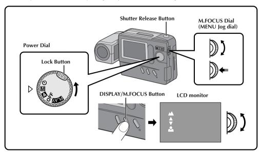
Turn the Power Dial, while pressing its Lock Button, to "M" or "S".
